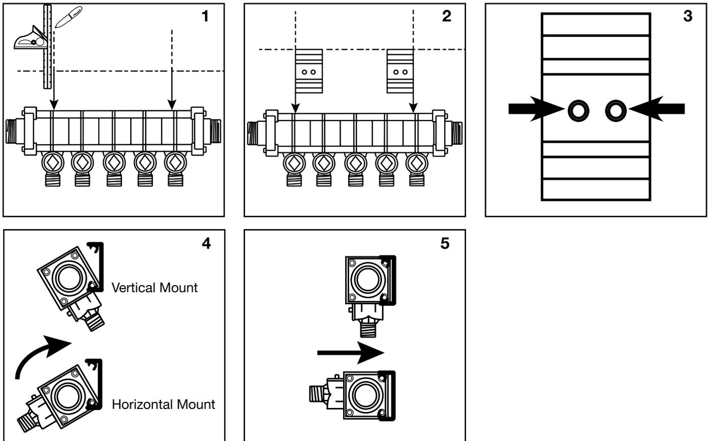
1. For proper bracket spacing, measure distance between the center ribs of the first and last MINIBLOC module. Mark this distance on the selected mounted surface.
